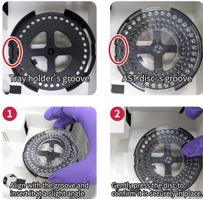
▲ Figure 3.4-2 Diagram of AST disc installation
