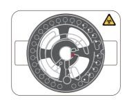
Place the reagent disc and tray rack into the instrument, close the lid and start testing according to the instructions.
