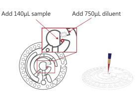
Use a pipette to inject 140µLsample into red circle and 750µL diluent into white circle
