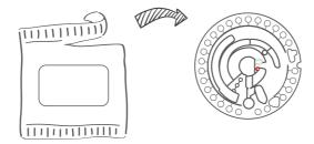
Take refrigerated disc out and warm it for 10 minutes at room temperature. Then, take the disc out of the sealed bag.
